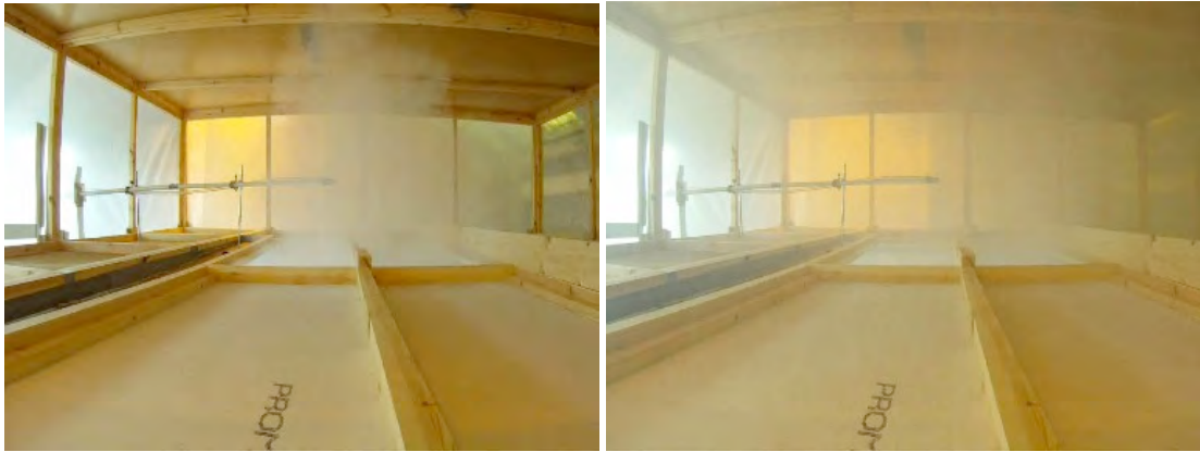
Figure 5.5 Screen shots from a video showing ceiling tile removal from a sealed void at a ventilation rate of 8 ach, 10 s after tile removal (left) and 3 minutes after tile removal (right)
