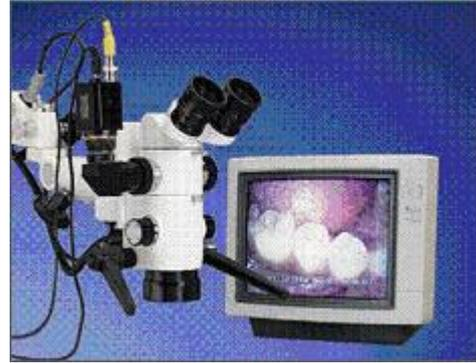
This is achieved by a **beam splitter** which is an optical device that splits a beam of light in two. The beam can be split 50:50 or 20:80. One portion of the beam is diverted to the eyepiece and the other to a camera or the assistant viewing eyepiece.
