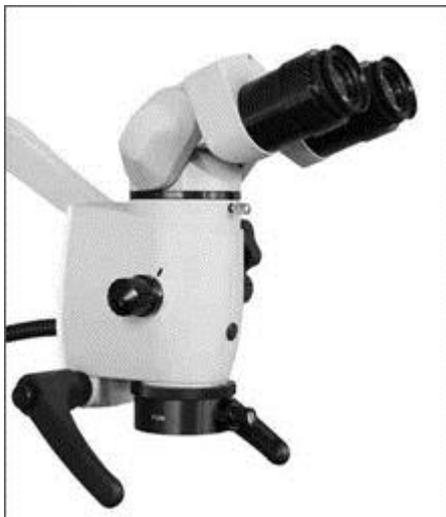
Surgical Operating Microscopes are stereo-microscopes. This means that there are two separate optical paths for the left and right eyes which view the operative field at slightly different angles. This gives excellent three dimensional vision (stereoscopic vision) and is ideal for work that involves fine dissection and movements such as microsurgery.
