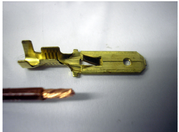
Strip and twist the wire to suit the terminal.
