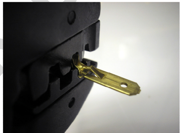
Crimp Section should line up with front jaw of crimp tool.
