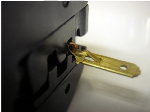
Insert wire into crimp terminal.
