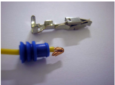
3. Bend copper wire
